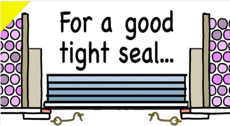
Attic Hatch Latch Attic Hatch Latch The goal is to match the R-value of the hatch to the overall attic R-value. Upgrading the weather stripping & installing a latch to the hatch will help compress the gasket & improve the attic hatch seal.
